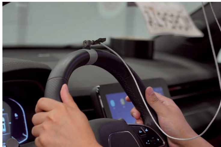
An 8763B accelerometer from Kistler is mounted on a steering wheel for NVH testing at the China Automotive Engineering Research Institute (CAERI) in Chongqing.
